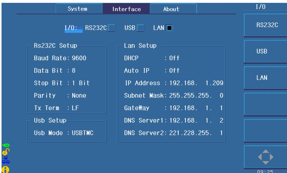
Figure 6-10 Network parameters of ST2883
